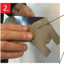
Use sand paper to aggressively sand down the edges of the end cap and where the end cap connects with the coating edge.
