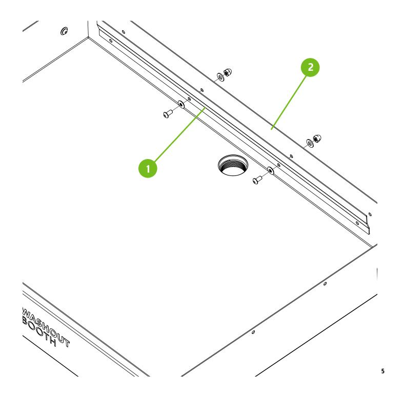
Install the side panels **(1)** to the main sink body **(2)**. Fully tighten the hardware. Neobond washers are inside of the sink and standard flat washers are outside of the sink.
