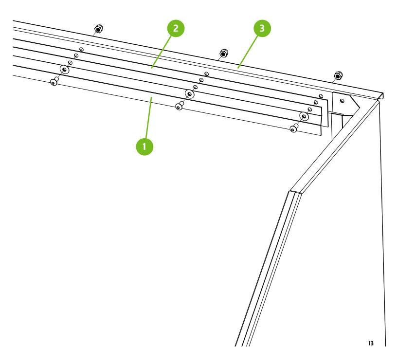
Install the final hardware in the upper corner of the side panels. Fully tighten the hardware at this time. After all hardware is tight, use supplied caulk to seal up all seams where water could leak. Allow to dry per caulking instructions.
