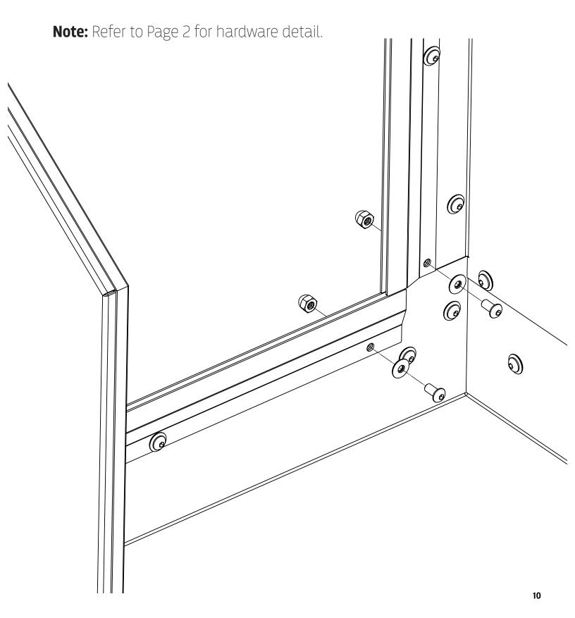
Attach the upper cross bar (1) to side panel (2) with the suppled hardware. DO NOT full tighten the hardware at this time. No flat washers are in lower hole.
