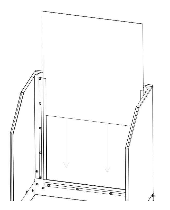
Attach the 26-3/8" upper back panel bracket (1) & upper spacer (2) to the top cross bar (3). Fully tighten the hardware at this step. Spacer is between the back acrylic panel and the top cross bar. No flat washers this step.
