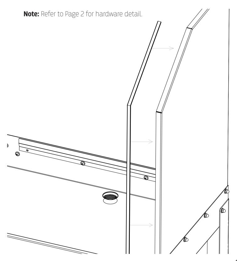
Install the 30-3/8" side rear panel brackets (1) to the side panels of the washout sink (2). DO NOT fully tighten hardware at this time. Omit the upper and lower hardware at this step. Neobond washers on the inside of the sink and the standard flat washers are on the outside.
