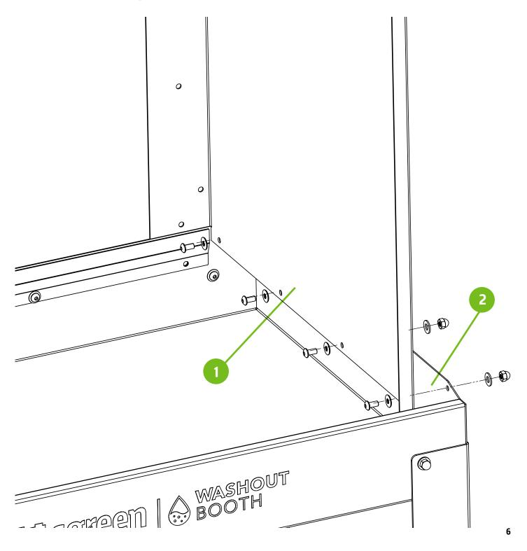
Partially attach the rear gussets (1) to the main sink body and side panels (2). NOTE: Only attach the two places shown in the drawing below.
