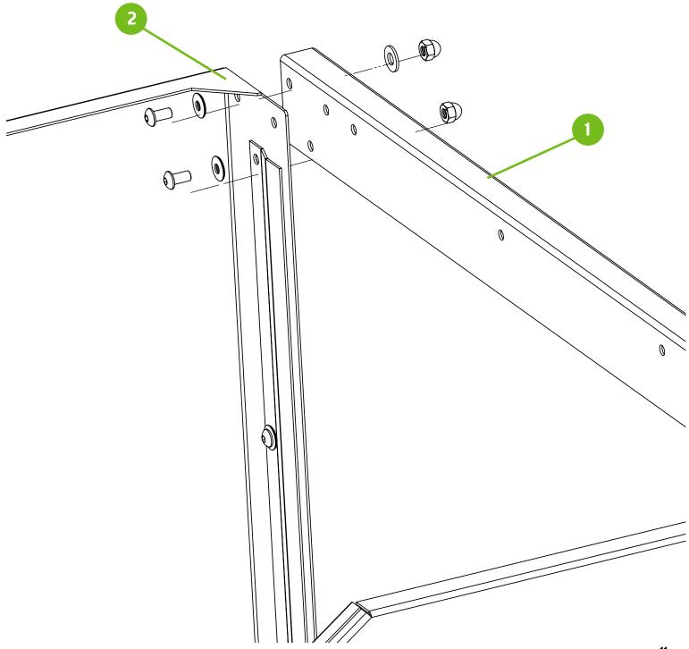
Slide the rear panel of the washout booth into the channels between the brackets and the side panels. Push down into the lower bracket. Align the top of back panel with the top edge of the side holding brackets. Fully tighten all loose hardware from the previous steps.
