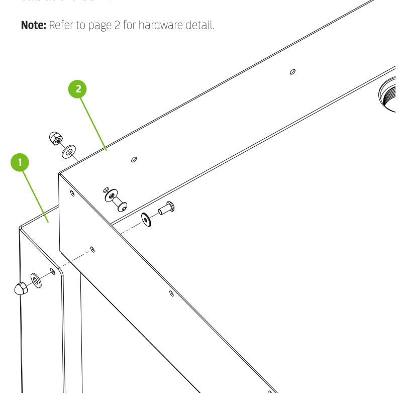
Install the 27-7/8" lower rear panel bracket (1) to the main sink body (2). Only attach the center 2 holes at this time. Do NOT fully tighten at this step. Neobond washers are inside of the sink and standard washers outside of the sink.
