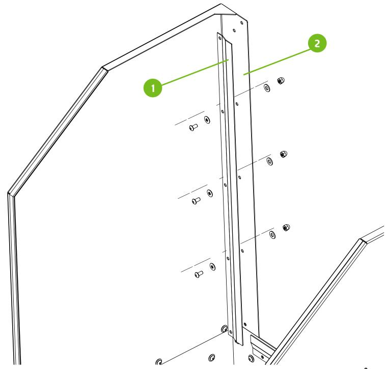
Install the lower rear corner hardware to the back panel holding brackets. **DO NOT** fully tighten the hardware at this time. No flat washers in this step.
