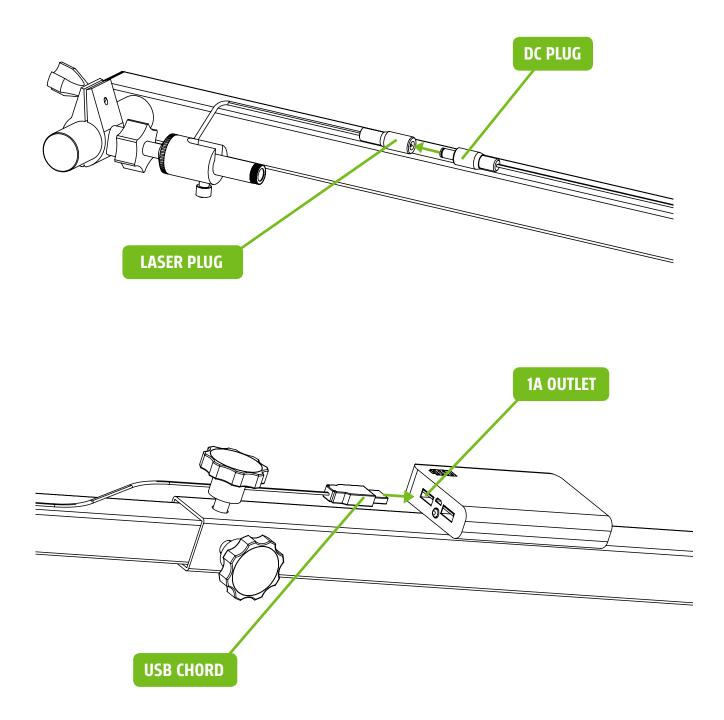
To adjust the clamp on the 1" post loosen knob (1), move into desired location and retighten. To adjust the swivel of the laser holder loosen knob (2), pivot into desired location and retighten. To adjust the focus of the laser cross hair use the end of the laser to get crisp line.
