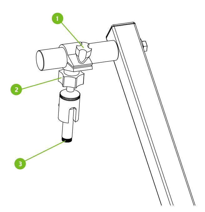
The upper tube is telescopic. To adjust the overall length of the assembly loosen the knobs (1), adjust to the desired location and retighten. The lower tube assembly pivots up and down by loosening knob (2). Once it is at the desired angle, lock down the lever tightly.
