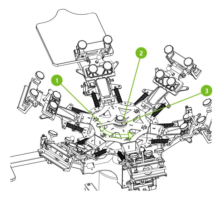
Install the Lower pivoting assembly (1) in place of the top washer removed from the previous step. Install the N10 nut (2) by hand to start to ensure that threads do not get damaged. Finally tighten the N10 nut with the supplied spanner wrench (3).
