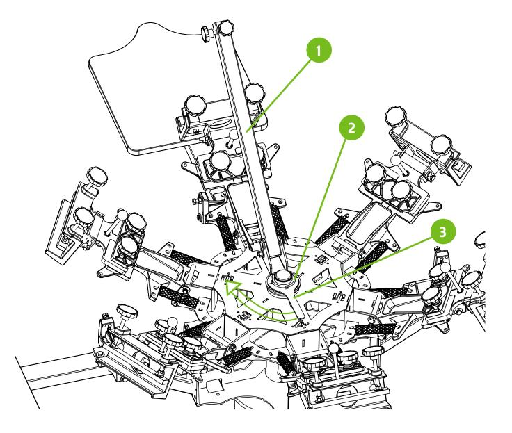
Install the Laser attachment with the supplied hardware to the upper telescoping tube. One 1/2" wrench is required for this step.
