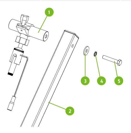
Loosen the lock-down knobs (1) and insert the upper telescoping tube into the lower pivoting tube assembly. Once the tube is installed, hold in place with the lock-down knobs.
